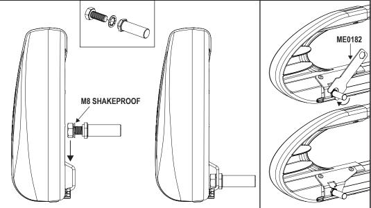
Assemble the roller spigot, M8x20 hex bolt and M8 shakeproof washer together. Place the assembly into the roller. Slide the roller onto the spigot fitted in step 14 and drop the other end into position. Tighten using the supplied tool.
