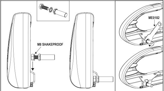
Assemble the roller spigot, M8x20 hex bolt and M8 shakeproof washer together. Place the assembly into the roller. Slide the roller onto the spigot fitted in step 12 and drop the other end into position. Tighten using the supplied tool (ME0182).
