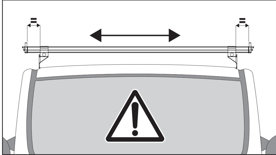
**6** Tighten the M8 flange nuts.
