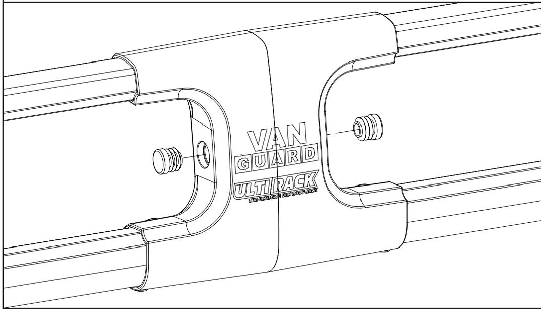
**15** Check bars are fully secured.
