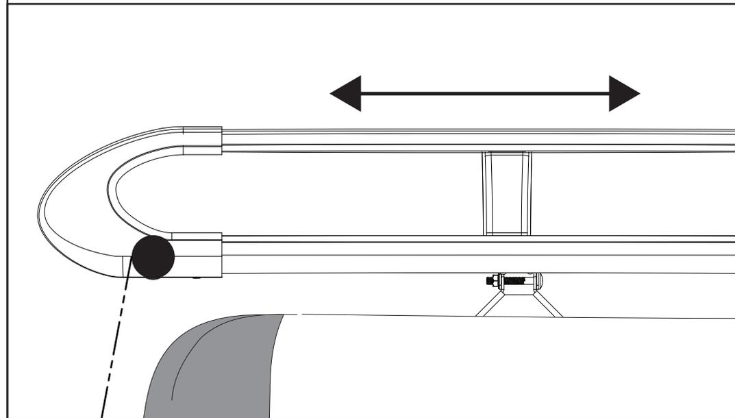
**10** Push on the lever to secure the 2X fixed roof bars into position.
