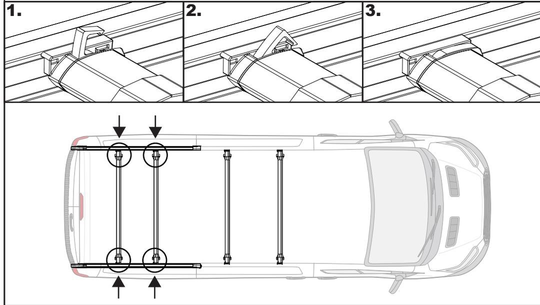
**9** Lift the front side rail sections into position (A1 & B1). Ensure that the side rails are connected to the roof bars correctly as per step 6.3.
