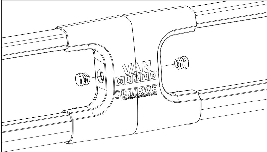
**16** Check bars are fully secured.
