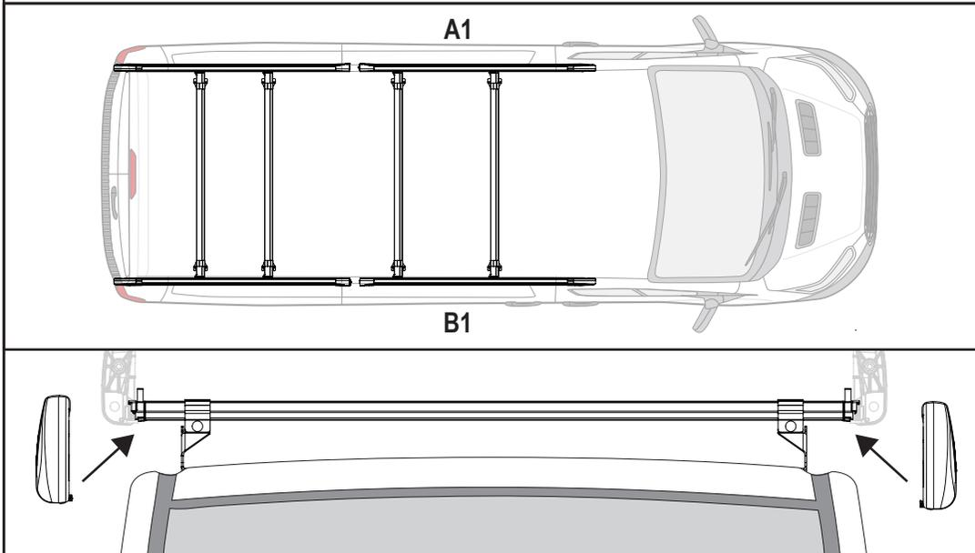
**10** Slide the front side rail upto the rear side rail and secure together using 1X M8x40 button bolt. Tighten using the supplied tool (FX4008). Repeat for the other side.
