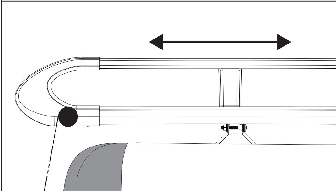
**8** Push on the lever to secure the 2X rear fixed roof bars into position.
