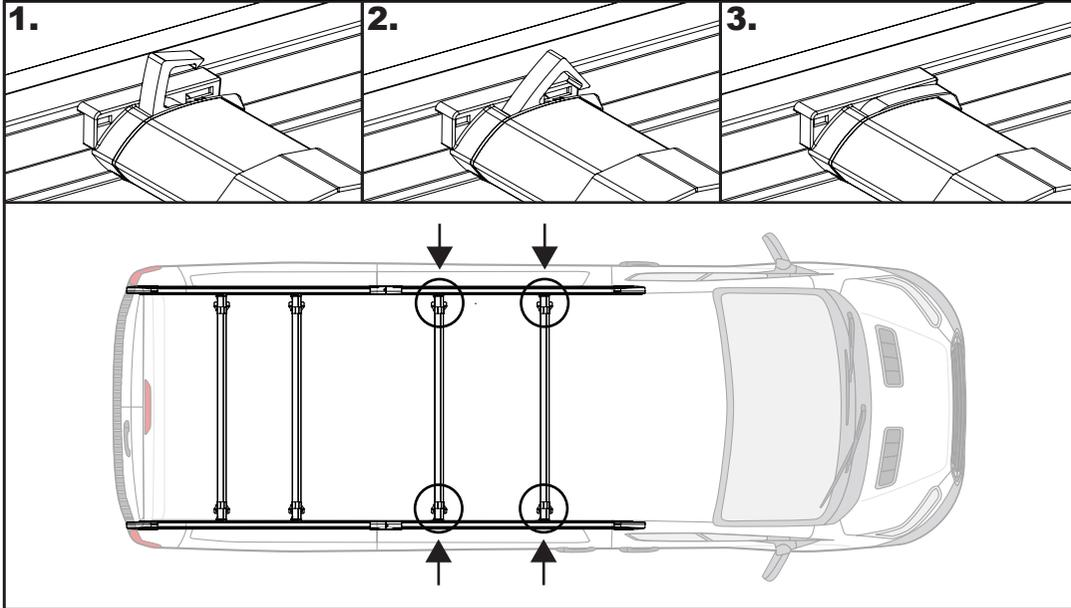
**12** Place the remaining roof bars into position. See page 2 for the recommended distances between the roof bars. Once in position push on the lever to secure in place.
