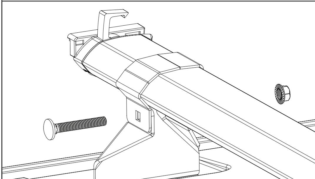
**4** Adjust the roof bars to ensure that they're evenly spaced on the vehicle.
