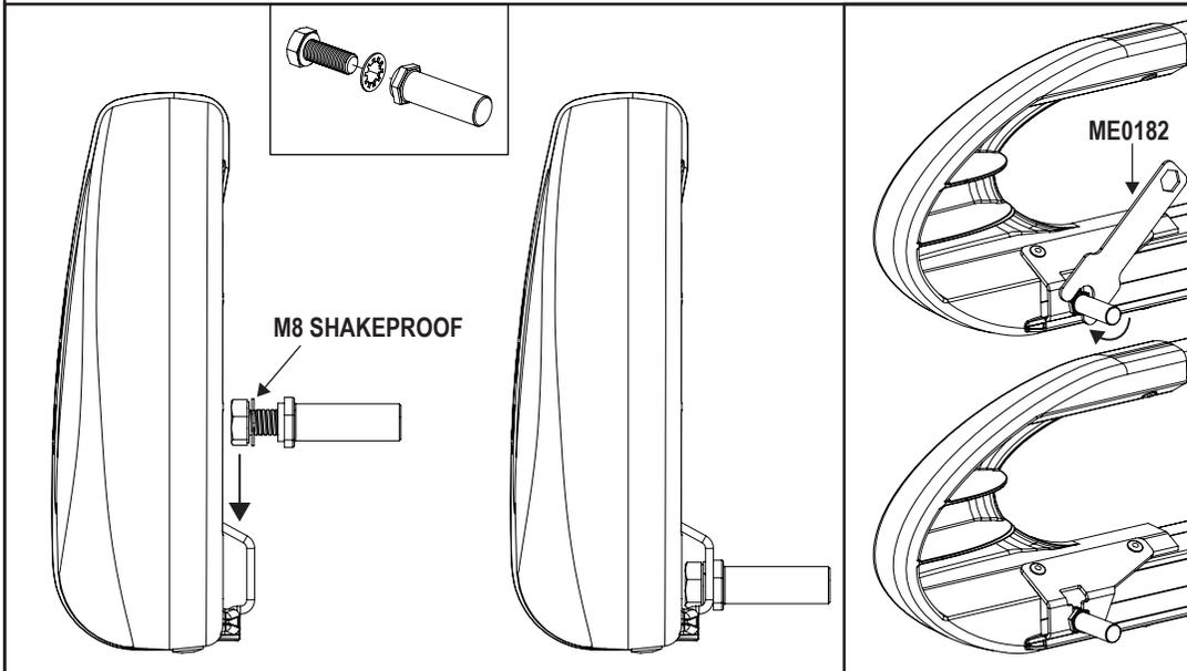
**14** Assemble the roller spigot, M8x20 hex bolt and M8 shakeproof washer together. Place the assembly into the roller. Slide the roller onto the spigot fitted in step 13 and drop the other end into position. Tighten using the supplied tool (ME0182).
