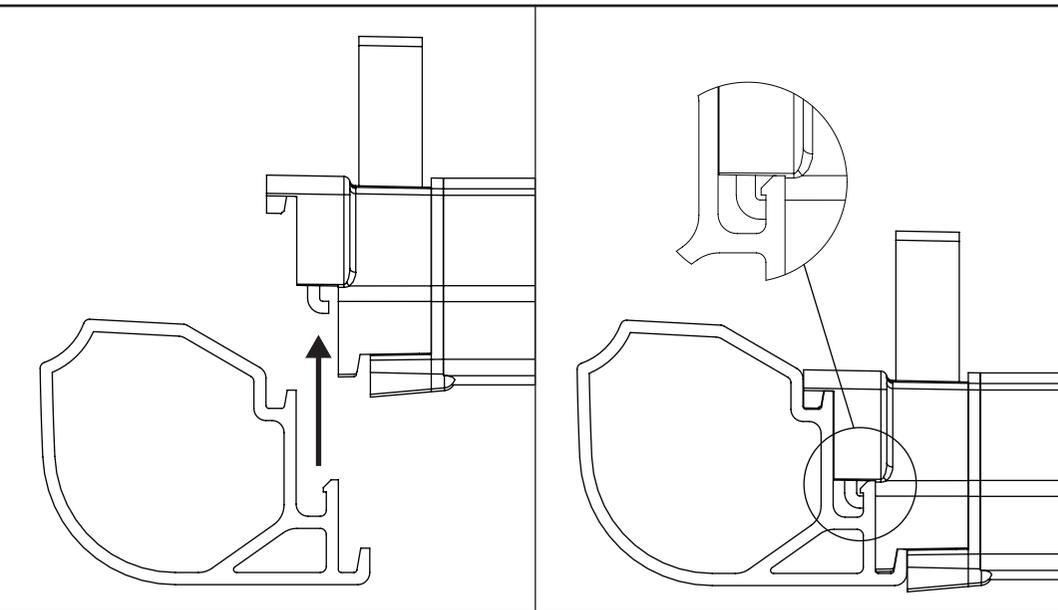
**7** Adjust the position of the rear side rails to suit the rear roller.
