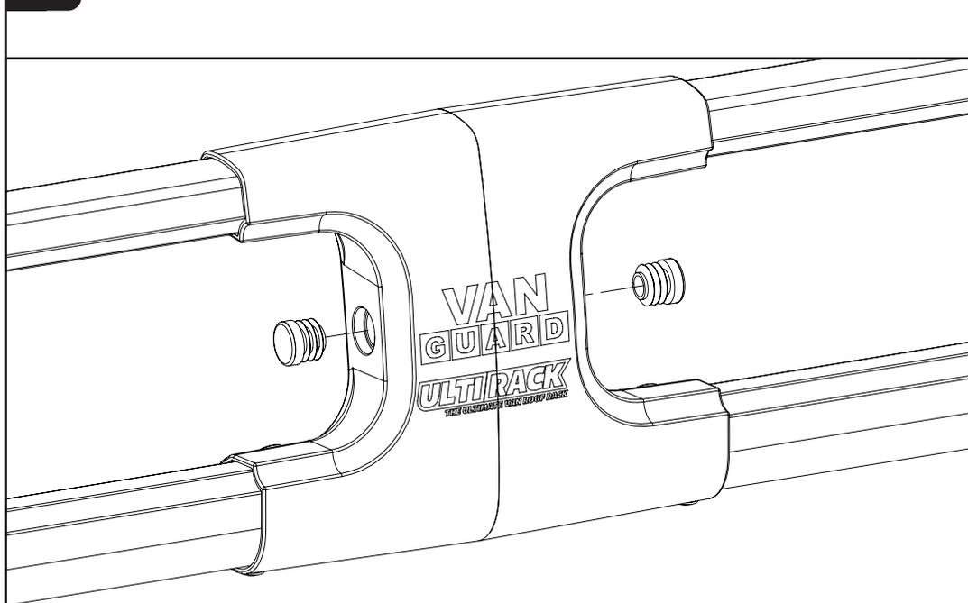
**14** Check bars are fully secured.
