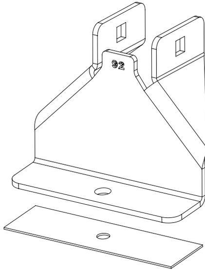
**2** Remove roof plugs to reveal the vehicles fixing points. Secure the roof brackets to the fixing points using M8x25 hex bolts, M8 shakeproof washers and M8 washers.
