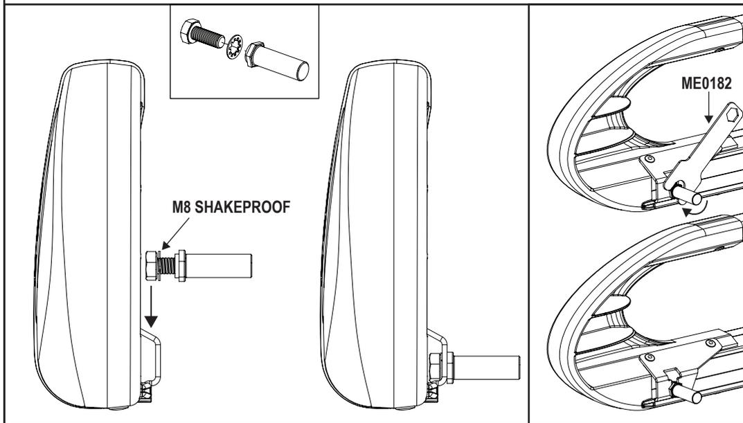
**12** Assemble the roller spigot, M8x20 hex bolt and M8 shakeproof washer together. Place the assembly into the roller. Slide the roller onto the spigot fitted in step 11 and drop the other end into position. Tighten using the supplied tool (ME0182).
