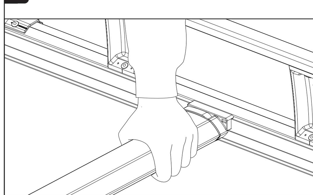
**15** Once fitted check fixings and parts to ensure they have been fully secured and tightened. Regularly check all fixings.
