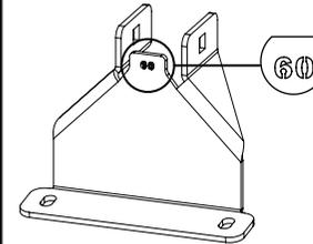
**2** Remove roof plugs to reveal the vehicles fixing points. Secure the roof brackets to the fixing points using M6x16 hex bolts, M6 shakeproof washers and rubber washers.
