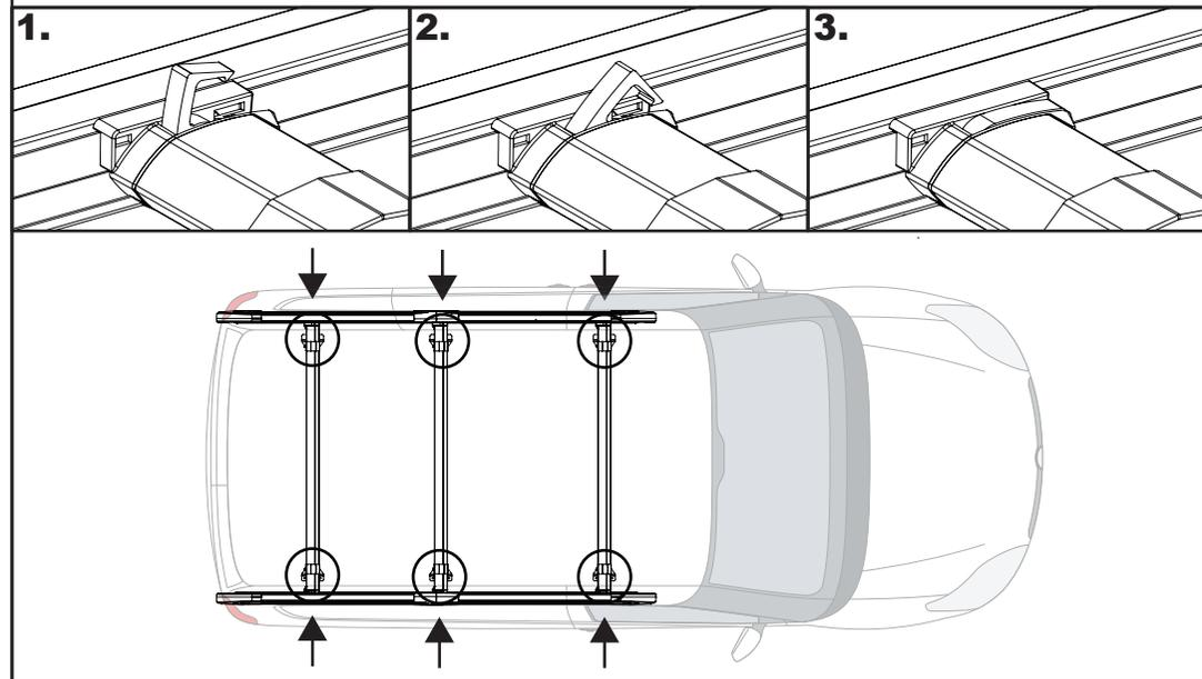
**10** Place the remaining roof bars into position. See page 2 for the recommended distances between the roof bars. Once in position push on the lever to secure in place.
