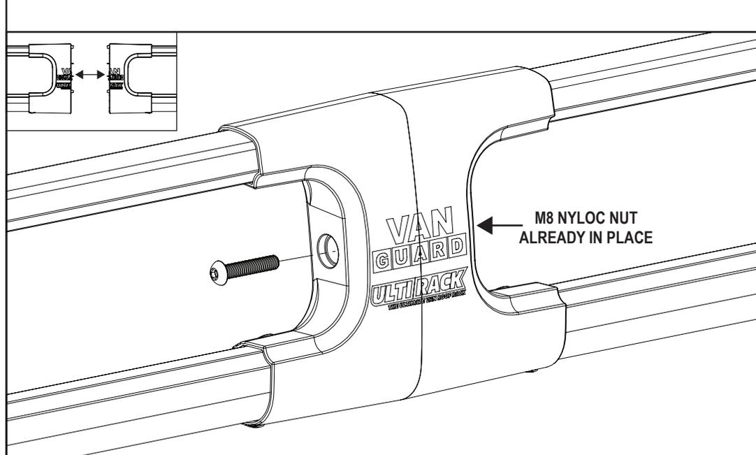
**7.1** Lift the side rails into position. Ensure that the side rails are connected to the roof bars correctly as per step 7.2.
