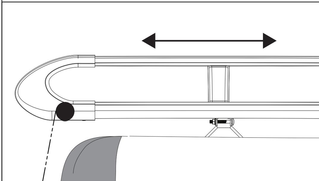
**9** Push on the lever to secure the 3X fixed roof bars into position.
