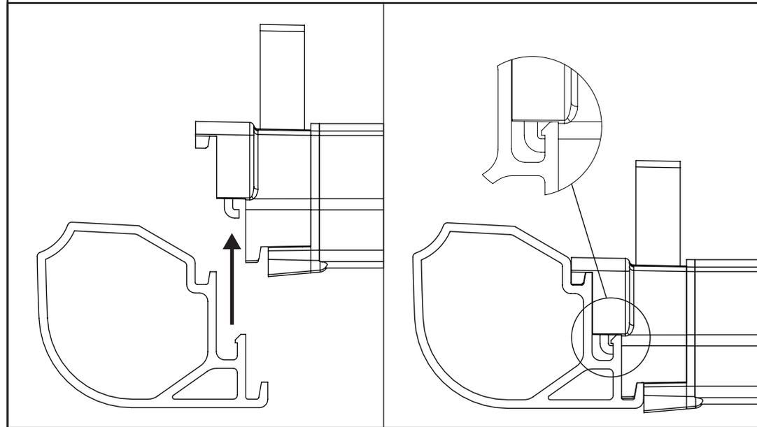
**8** Adjust the position of the side rails to suit the rear roller.
