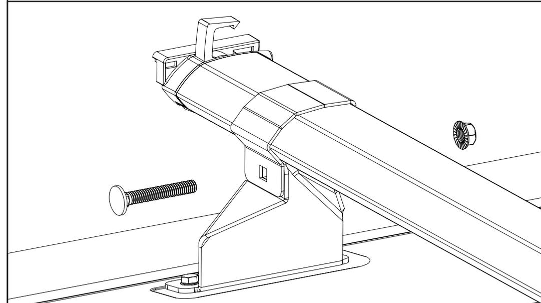
**4** Adjust the roof bars to ensure that they're evenly spaced on the vehicle.
