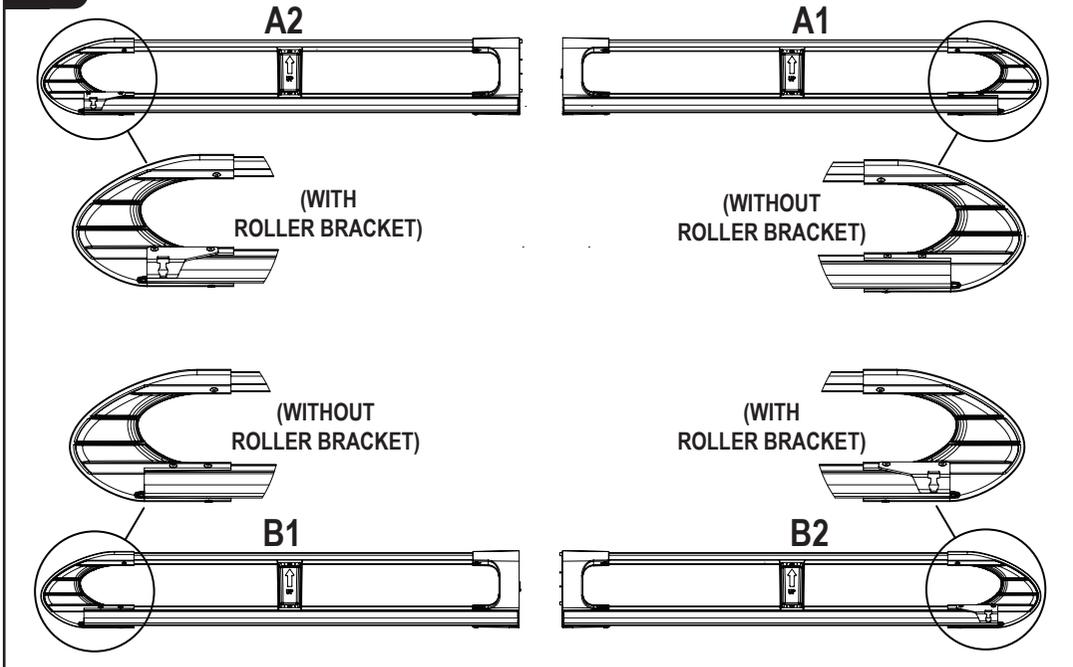
**6.2** Assemble the side rails together using 1X M8x40 button bolt. Tighten using the supplied tool (FX4008). Repeat for the other side.
