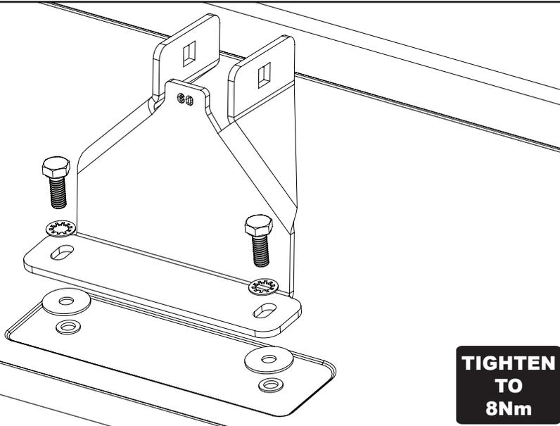
**3** Loosely secure roof bars to the roof brackets using M8x55 coach bolts and M8 flange nuts.
