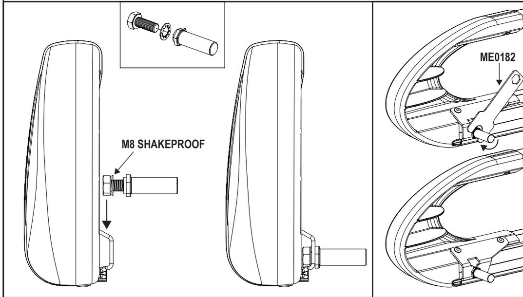
**12** Assemble the roller spigot, M8x20 hex bolt and M8 shakeproof washer together. Place the assembly into the roller. Slide the roller onto the spigot fitted in step 12 and drop the other end into position. Tighten using the supplied tool (ME0182).
