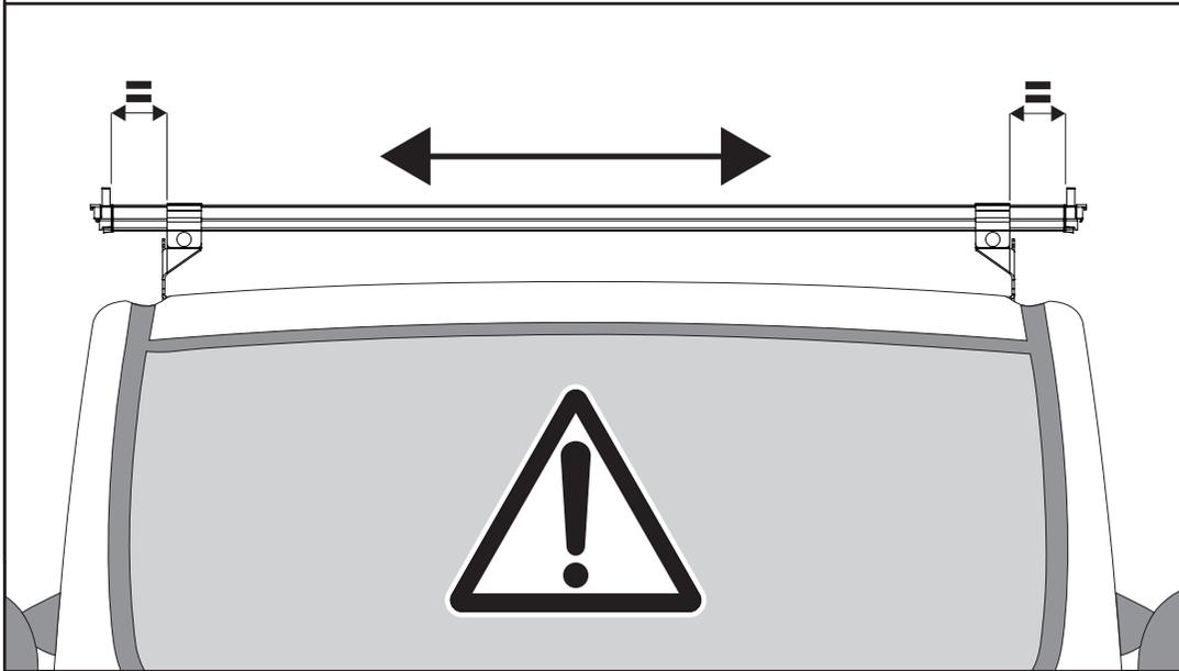
**5** Tighten the M8 flange nuts.
