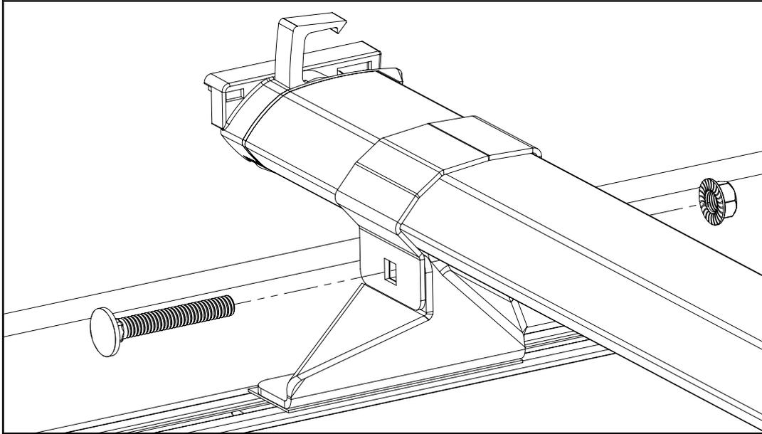
**3** Adjust the roof bars to ensure that they're evenly spaced on the vehicle.
