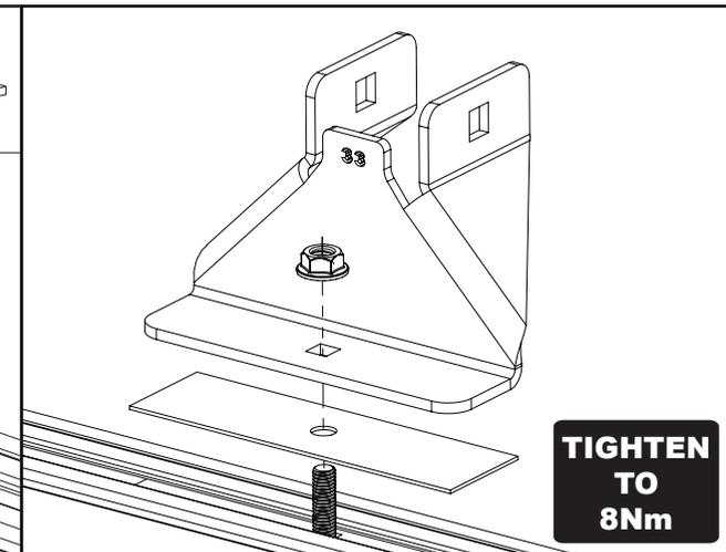
**2** Loosely secure roof bars to the roof brackets using M8x55 coach bolts and M8 flange nuts.
