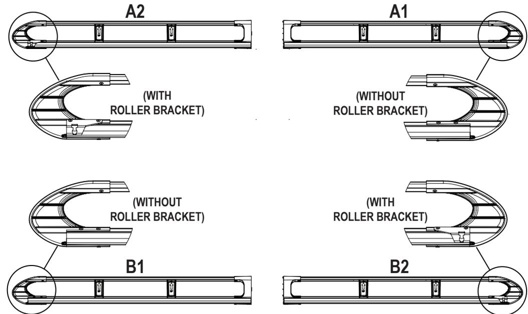
**5.2** Lift the rear side rail sections into position (A2 & B2). Ensure that the side rails are connected to the roof bars correctly as per step 5.3.
