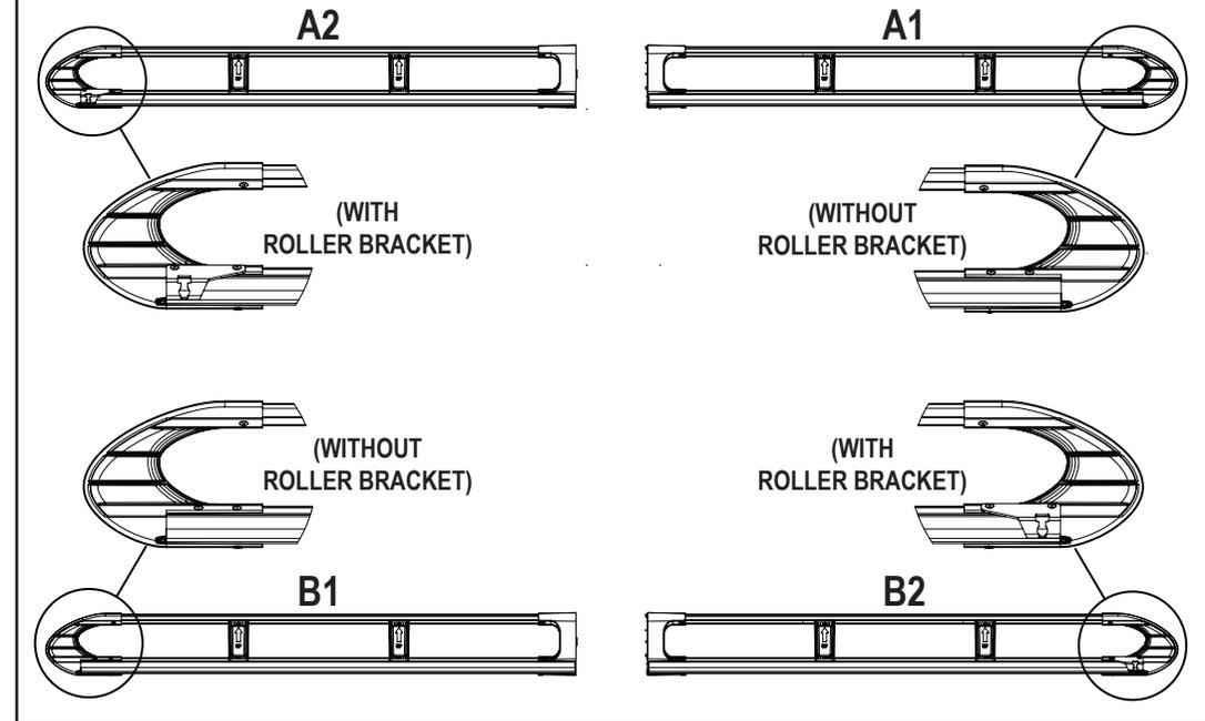
**7.2** Assemble the side rails together using 1X M8x40 button bolt. Tighten using the supplied tool (FX4008). Repeat for the other side.
