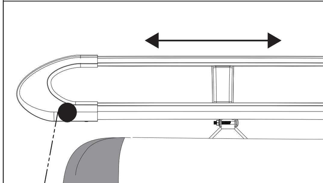
**10** Push on the lever to secure the 3X fixed roof bars into position.
