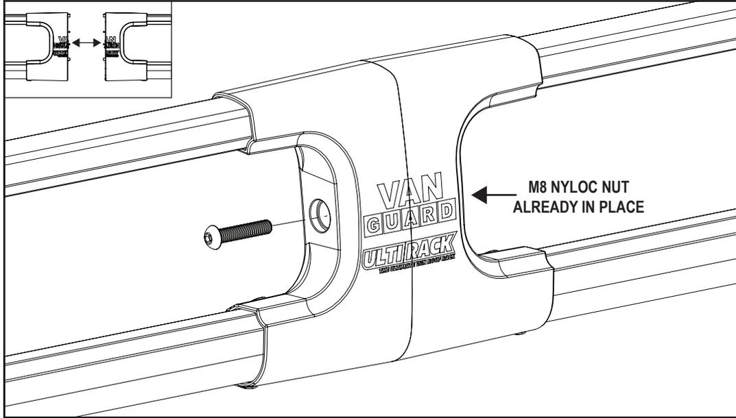
**8.1** Lift the side rails into position. Ensure that the side rails are connected to the roof bars correctly as per step 8.2.
