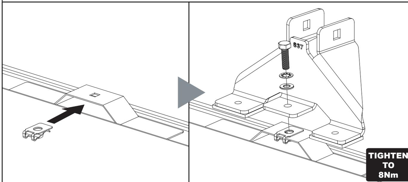
**4** Loosely secure roof bars to the roof brackets using M8x55 coach bolts and M8 flange nuts.
