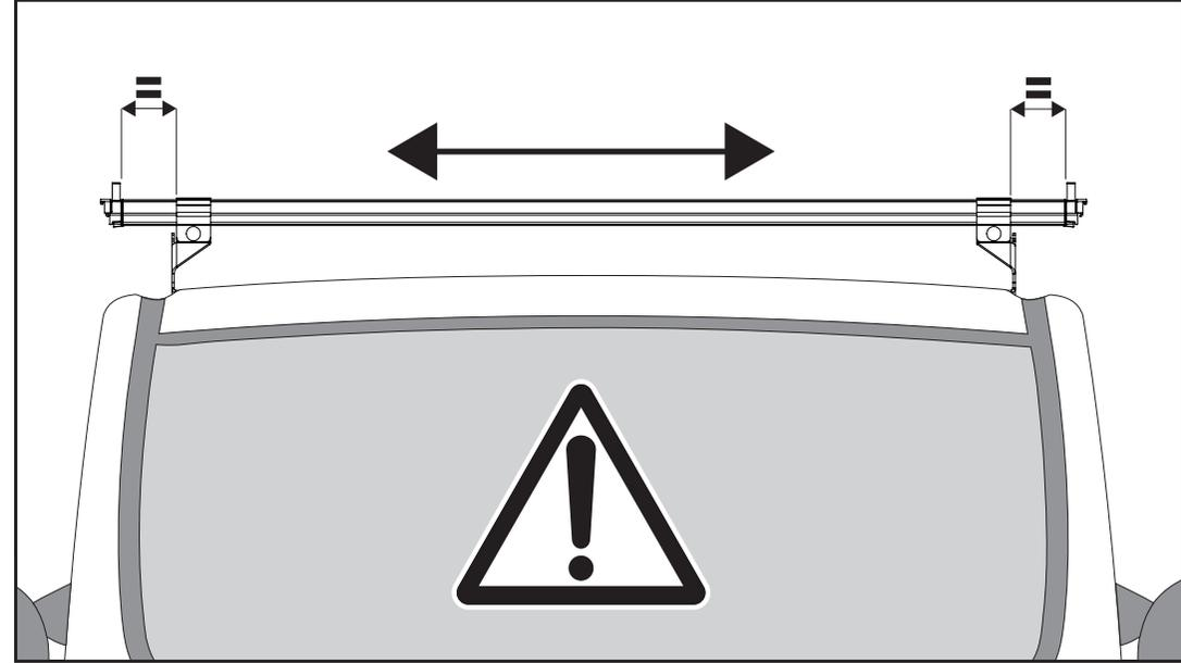
**6** Tighten the M8 flange nuts.
