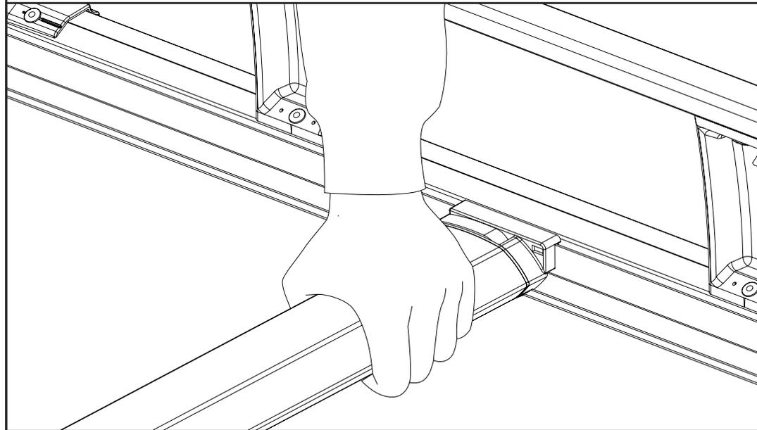
**16** Once fitted check fixings and parts to ensure they have been fully secured and tightened. Regularly check all fixings.
