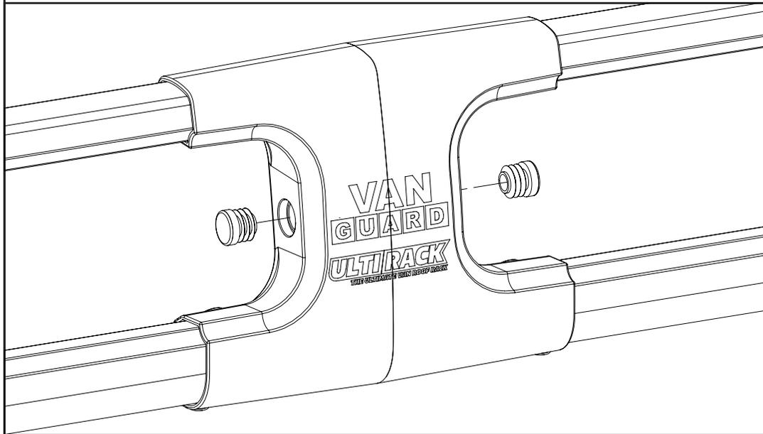
**15** Check bars are fully secured.
