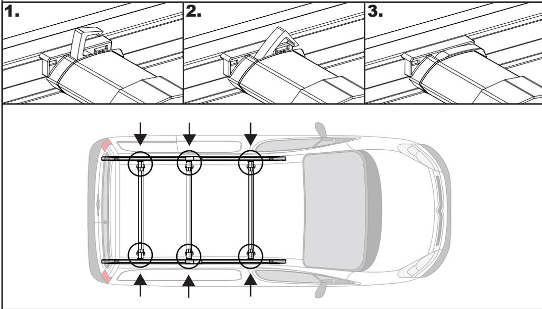
**11** Place the remaining roof bars into position. See page 2 for the recommended distances between the roof bars. Once in position push on the lever to secure in place.
