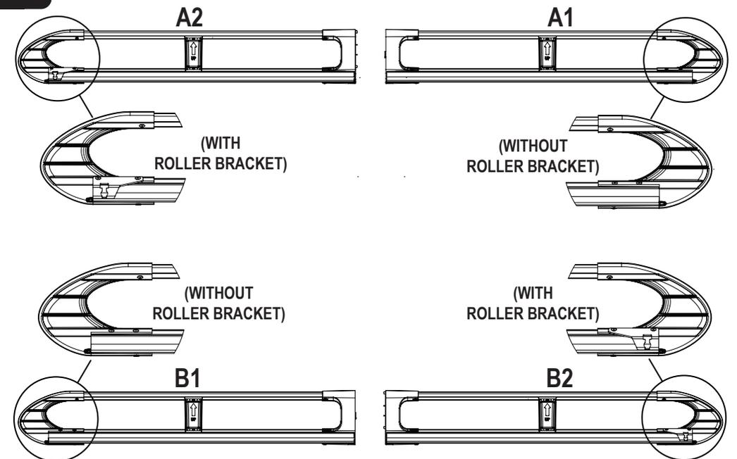
**7.2** Assemble the side rails together using 1X M8x40 button bolt. Tighten using the supplied tool (FX4008). Repeat for the other side.
