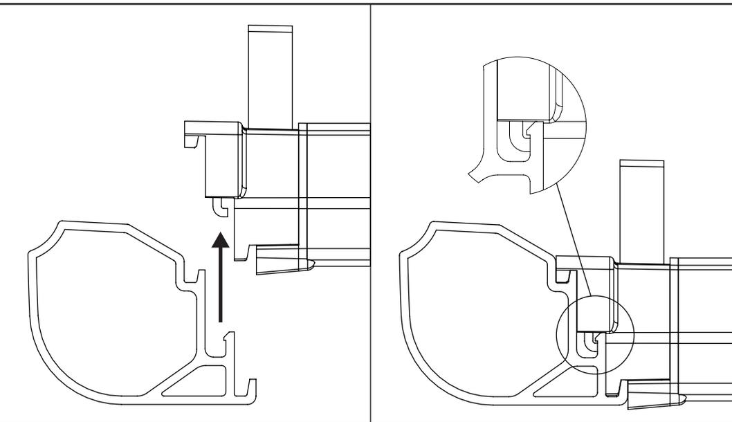
**6** Adjust the position of the rear side rails to suit the rear roller.
