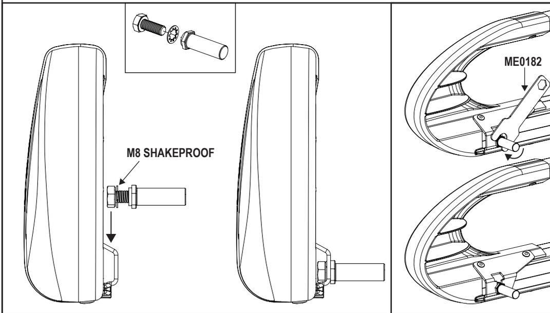
**13** Assemble the roller spigot, M8x20 hex bolt and M8 shakeproof washer together. Place the assembly into the roller. Slide the roller onto the spigot fitted in step 12 and drop the other end into position. Tighten using the supplied tool (ME0182).
