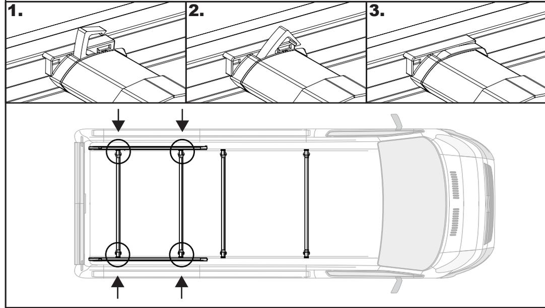
**8** Lift the front side rail sections into position (A1 & B1). Ensure that the side rails are connected to the roof bars correctly as per step 5.3.
