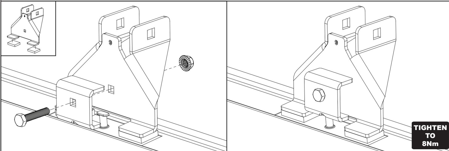
**2** Loosely secure roof bars to the roof brackets using M8x55 coach bolts and M8 flange nuts.
