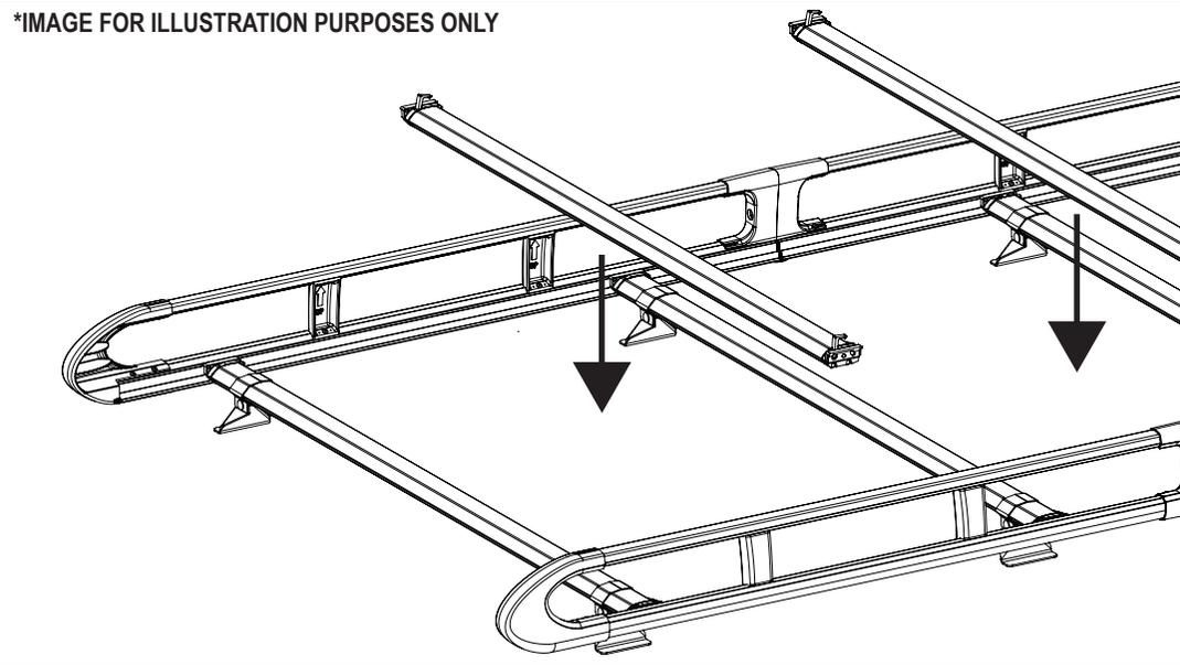
**12** Secure the roller spigot to the **left hand roller bracket only** using a M8x20 hex bolt and a M8 shakeproof washer. Ensure that the shakeproof is on the inside of the roller bracket and that the spigot sits flush / straight. Tighten using the supplied tool.
