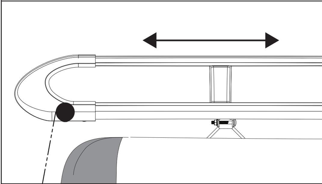
**7** Push on the lever to secure the 2X rear fixed roof bars into position.
