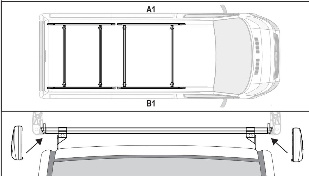
**9** Slide the front side rail up to the rear side rail and secure together using 1X M8x40 button bolt. Tighten using the supplied tool (FX4008). Repeat for the other side.
